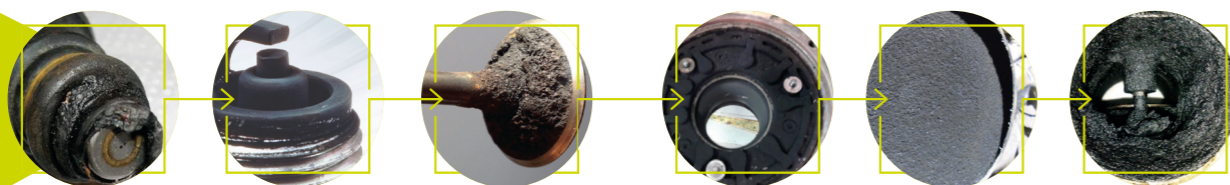
Injectors with soot Spark plugs with carbon deposits Carbonised valves Blocked turbo Obstructed FAP EGR with carbon deposits
