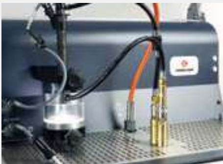
TESTING WITH ILLUMINATED SPRAY CHAMBER.
