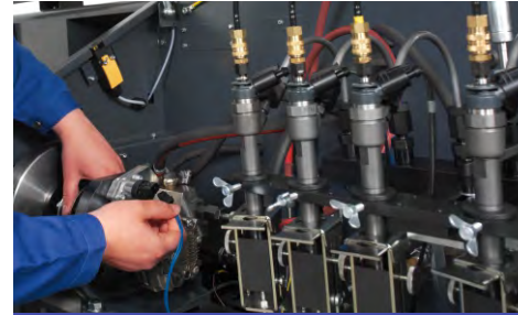
DIESEL FUEL INJECTION TESTING AND REPAIR
